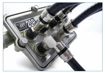
EX<sup>®</sup> Universal compression connectors used in combination with port seals ensure proper port sealing every time Right angle connectors prevent improper cable bending and tap ports from breaking in smaller pedestals
